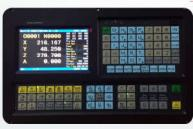
Controller based Lathe ARM9+FPAG large scale CPU processor ,7" TFT display, Meet 2 Axes lathe machine. this controller support ISO G codes, Macro program and PLC ladder, very flexible for unstandard function
